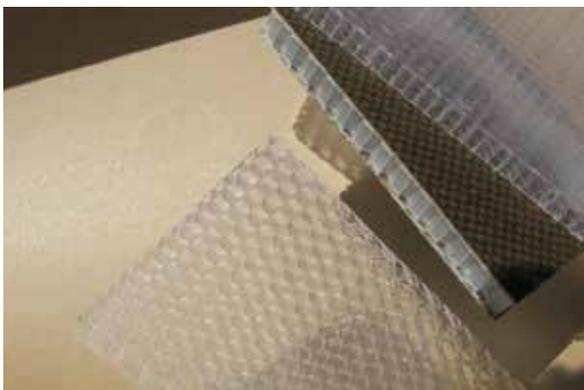
**EconCore is proud to present the first 100% bio-based composite panel. Recently EconCore has optimized the patented ThermHex production technology to produce honeycomb cores and sandwich panels made from bio-based plastics.**
